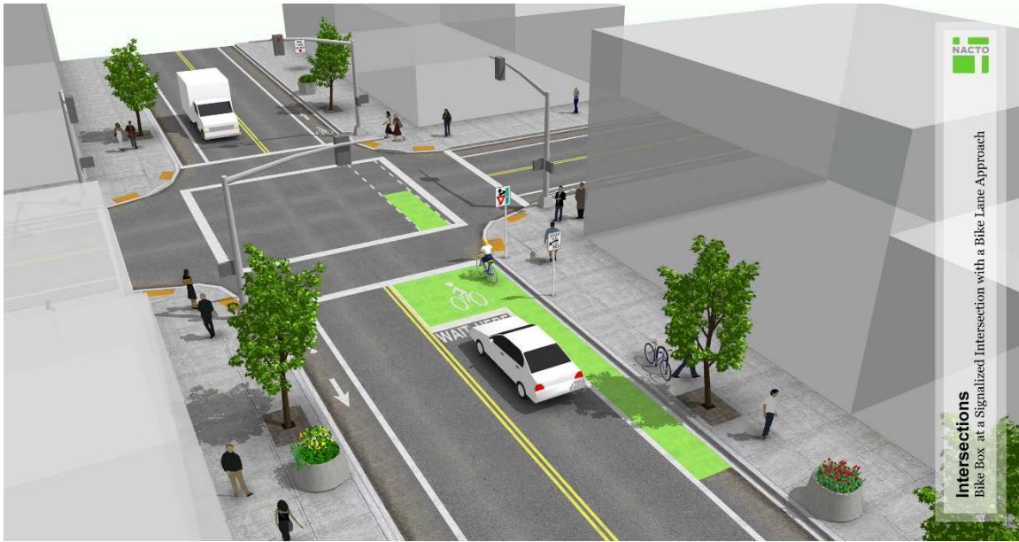
Figure 51 Example of a Bike Box at a Signalized Intersection with a Bike Lane Approach
